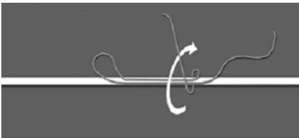
Roll one end of the thread around the loop (made of the same thread) and the string body
