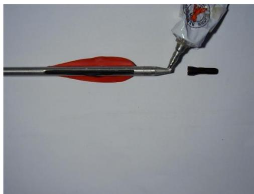
4. Press the nock onto the shaft and rotate it to spread the glue.
