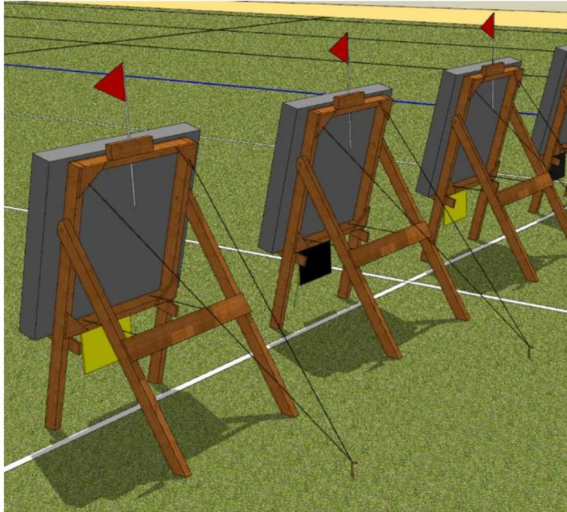
*Figure 11. Target Buttruss Rear View showing tie back*
