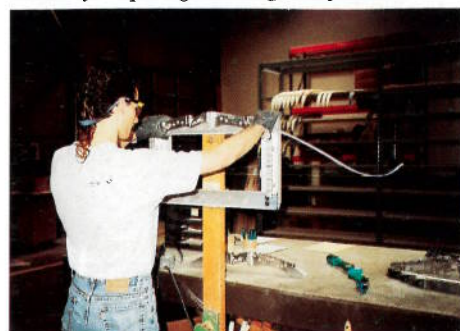
Tilting is very important in recurve bow production. Perfectly tilt bow can be still readjusted by an archer.
